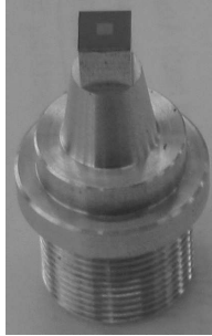
Fig. 1: Photograph of the target holder equipped with a thin SiN membrane as carrier foil for the ^{232}\text{Th} target spot.
