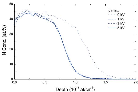
Fig. 1: Nitrogen concentration as a function of depth, measured with ERDA for ZrN films deposited at different pulse bias.
