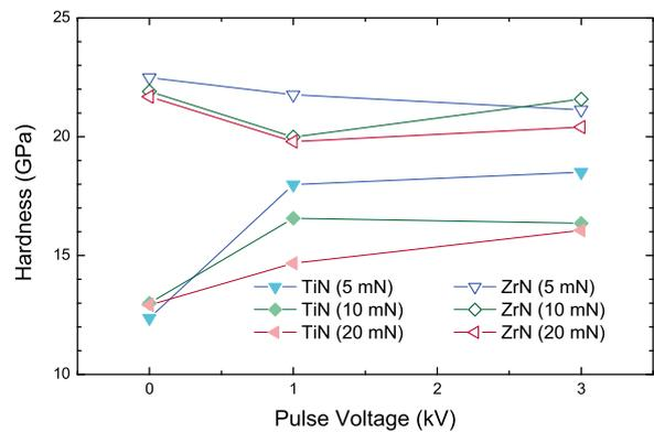
Fig. 2: Dynamic hardness, as measured with a Berkovich nanoindenter, as a function of applied load and deposition conditions.
