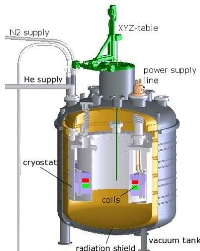
Fig. 2: CAD drawing of CoTex
