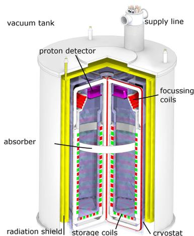
Fig. 1: CAD drawing of the PENeLOPE design
