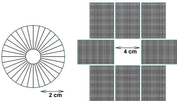
Fig. 1: Cut through the two silicon layers. Left: layer 1, right: layer 2. The hole in the middle is left for the beam.
