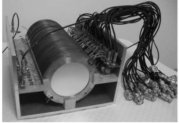
Fig. 1: PPAC array (25 targets) for the detection of fission fragments from <sup>232</sup>Th photofission.
