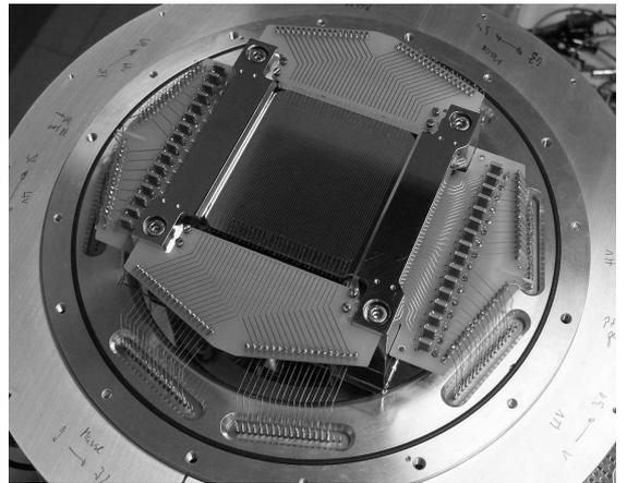
Fig. 2: 2D-segmented planar germanium Compton polarimeter, optimized for the detection of photons from Unruh (and Larmor) radiation with  $E_\gamma < 300 \text{ keV}$ .
