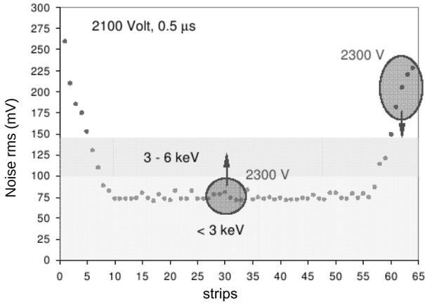
Fig. 4: Measured electronic noise level of all 64 strips on the high voltage side. The resolution is estimated by measuring the FWHM of a reference strip in the center region of the crystal.
