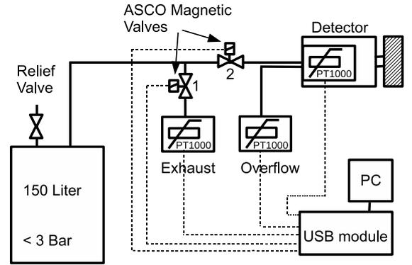
Fig. 5: Layout of the automatic LN2 filling system.
