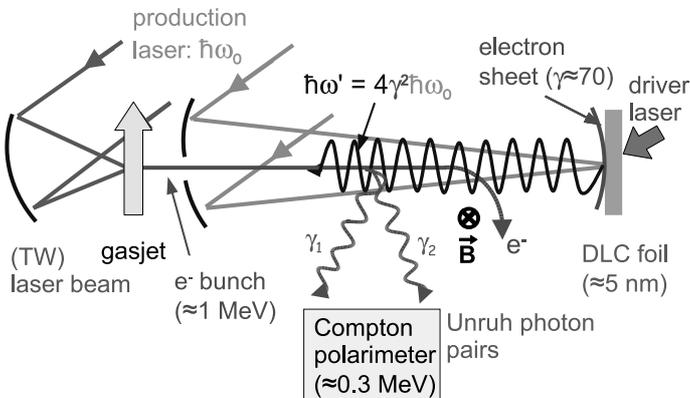
Fig. 1: Schematical view of an experimental setup for the detection of Unruh radiation originating from laser-accelerated electrons interacting with the strong periodic field of a counter-propagating X-ray beam.
