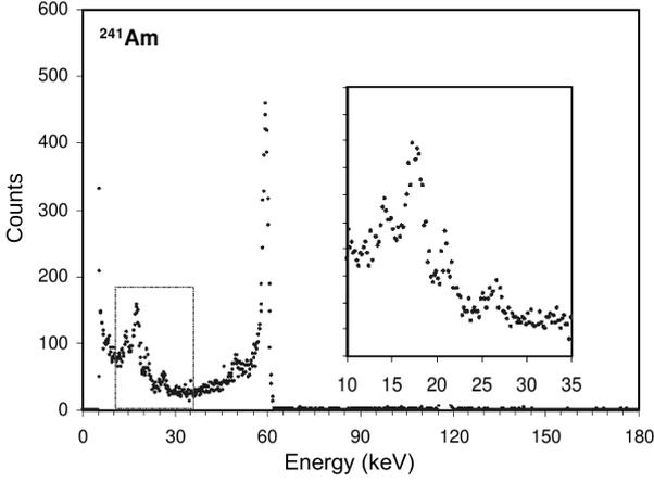
Fig. 3: Energy spectrum of a reference strip of the high voltage side in the center of the Ge crystal. Obtained from a  $^{241}\text{Am}$  source.
