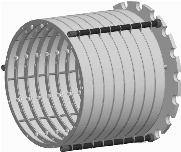
Fig. 2: Design of the eightfold-segmented DC electrode system for the cryogenic gas cell at SHIPTRAP.
