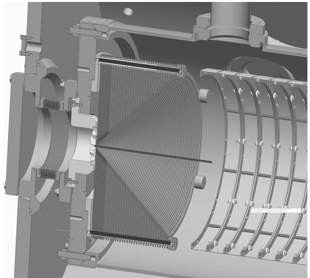
Fig. 4: Design of the RF (+DC) funnel system with 75 ring electrodes.
