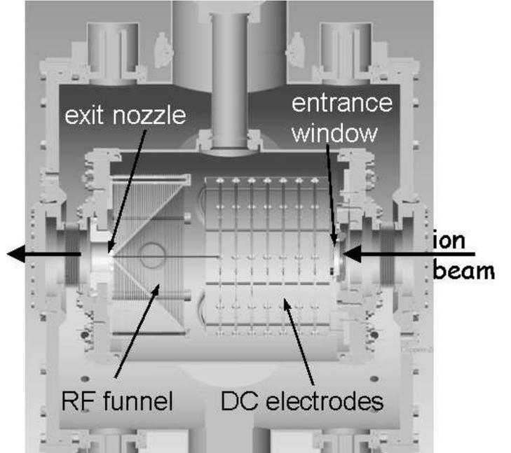
**Fig. 1:** Design of the cryogenic gas cell for SHIPTRAP with the cold inner part of the gas cell, isolated by an outer evacuated vessel. The inner part carries the extraction electrode system: the metallic entrance window, the segmented DC electrodes, the RF funnel and the extraction nozzle.
