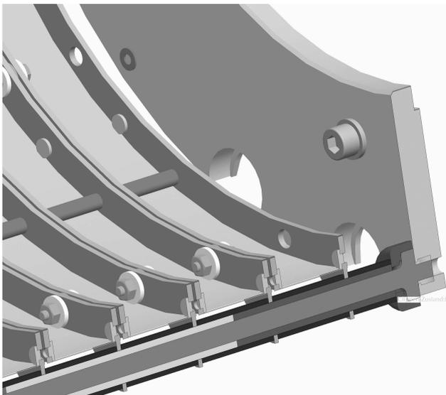
Fig. 3: Mounting of the segmented DC electrode system. The eight segments are supported by 3 steel rods (diameter 6 mm), which themselves are electrically isolated via ceramic tubes from the eye ring holders. The distance between the segments is preserved via ceramic spacers.
