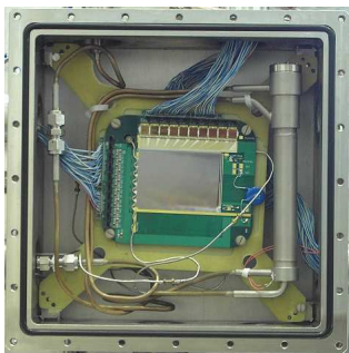
Fig. 2: Photograph of a fully equipped cryogenic beam station. The phase separator and one detector module are visible. The silicon wafer is glued between two L-shaped PCBs, holding the APV read-out chips and the pitch adapters, which are visible here for the side with 1280 strips read out by 10 APVs.
