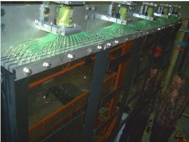
Fig. 1: View from above on the 5 upper detector blocks of the Sandwich Counter showing the bundles of 1 mm light guide fibres emerging from the 5 scintillator layers per block and ending in plastic cylinders for photomultiplier attachment. The scintillators (total thickness: 4cm) are stacked together with 7-mm steel-covered lead plates.
