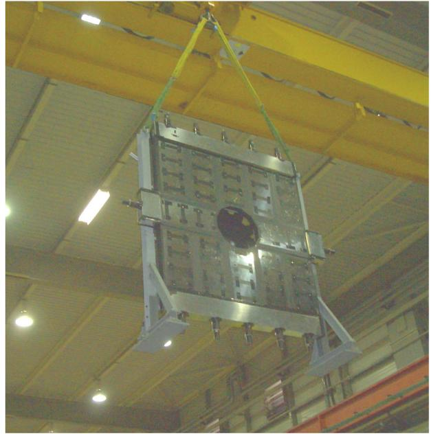
Fig. 2: View of complete detector with  $2.5 \times 3 \text{ m}^2$  support frame during craning. The 12 photomultiplier rears are seen sticking out of the light shielding boxes covering the light-guides.
